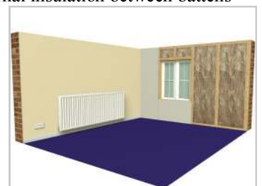
Internal insulation between battens
