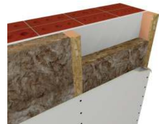
Internal insulation between battens
