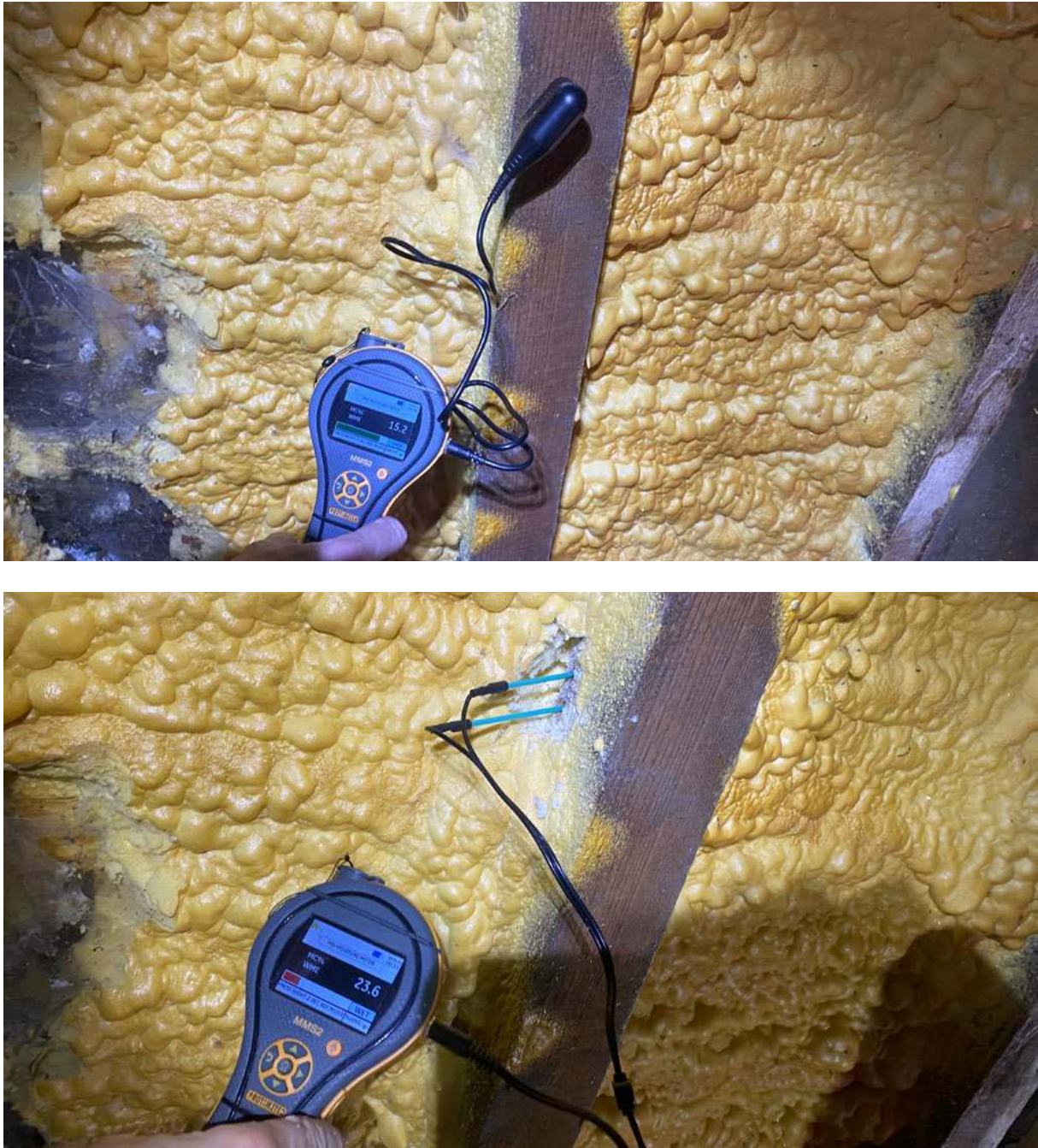
Figure 3: Spray foam insulation can make it difficult to identify problems to the roof because the timbers can be 'dry' on their exposed, visible surface but 'wet' behind the spray foam
